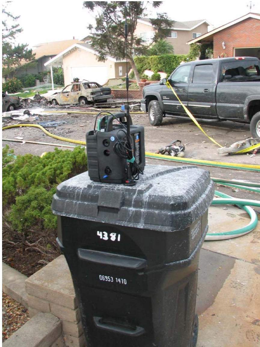
Photograph 4: Air monitoring equipment during clean up activities.
