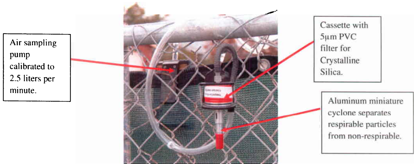
Figure 3. Dust sampling for Metals, Asbestos and Silica at the site fence line (Location D).
