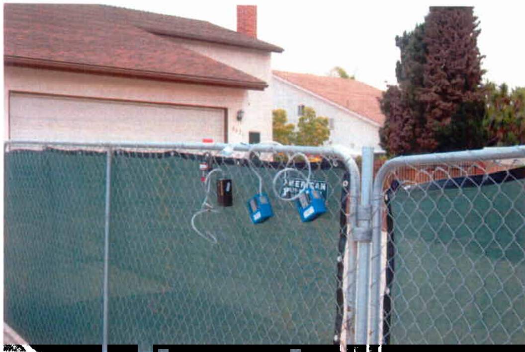
Figure 3. Dust sampling for Metals, Asbestos and Silica at the site fence line (Location D).
