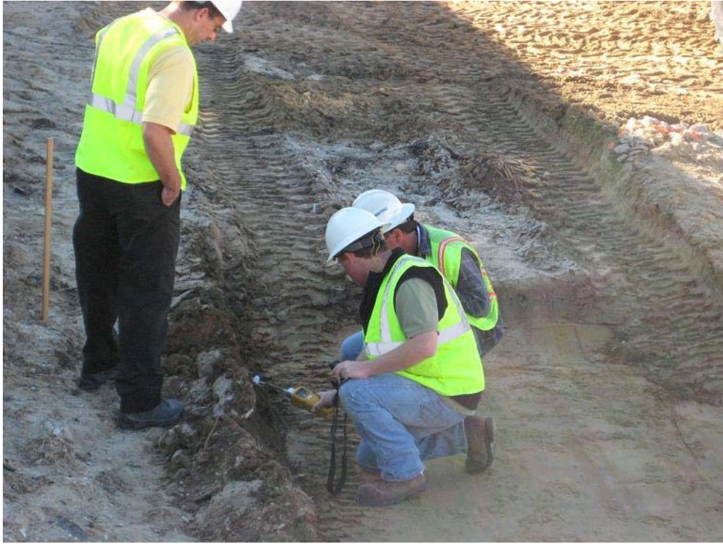
Photograph 3: Monitoring for organic vapor in soil using a photo ionization detector.
